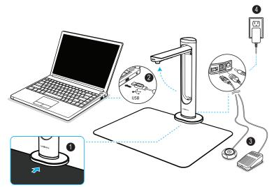
NOTE: Ensure the scanning pad is in contact with the scanner base.
